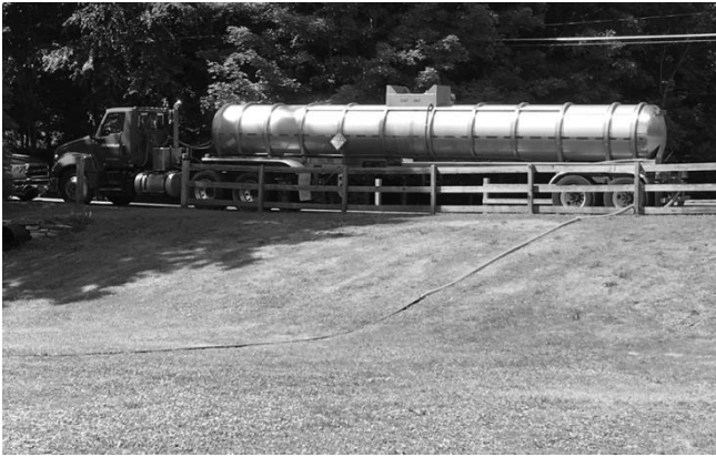
Fig. 1 Tanker Pumping PAC to the Tanks at the Shore
